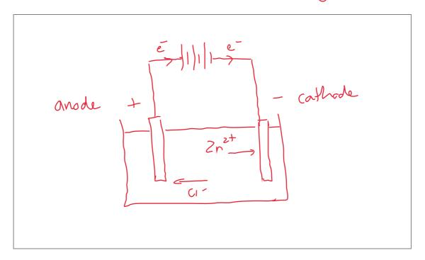
As the cell operates, a grey solid deposits on the surface of one of the electrodes and bubbles of a greenish yellow gas form on the surface of the other electrode.
