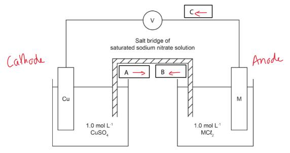
It was observed, that over time, the unknown metal electrode reduced in size and the solution containing  $MCI_2$  remained colourless.
